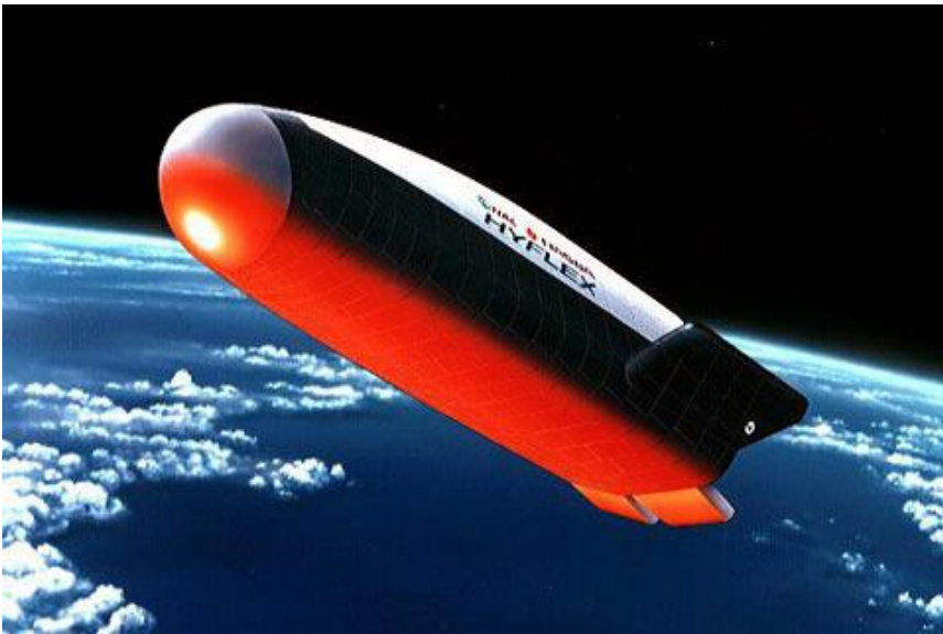
Fig. 10.2: JAXA HYFLEX Lifting Body Uncrewed Hypersonic Re-entry Experimental Vehicle (Image Courtesy of JAXA)
