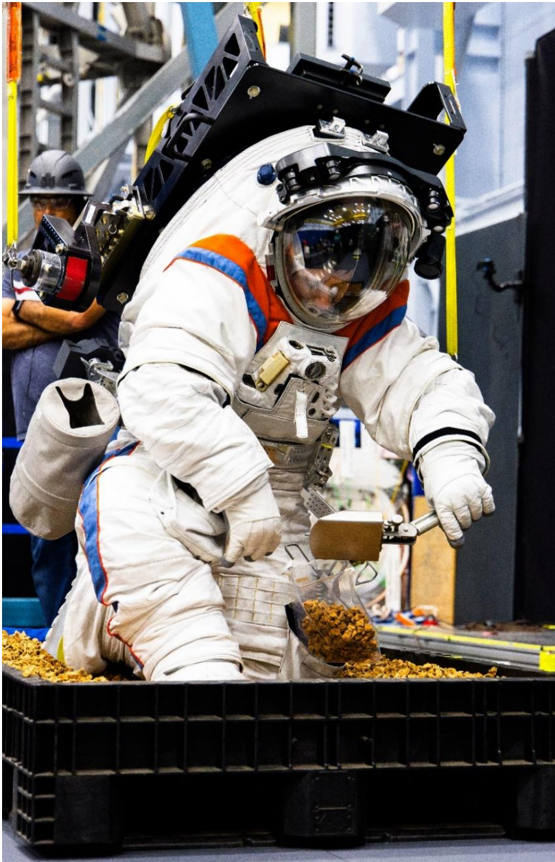
Fig. 5.4; The Axiom Space developed axEMU Space Suit under Testing at the Johnson Space Center (Image courtesy of NASA)
