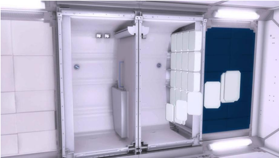
Fig. 6.3: NASA Design for Astronaut “Storm Shelter” for Radiation Protection (Source: NASA)
