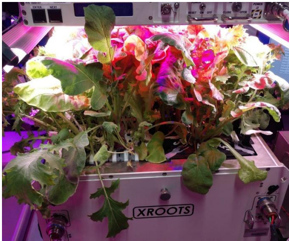
Fig. 5.2: XROOTS aeroponic test bed facility on board the ISS
